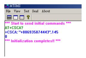
If the message "\*\*\* Initialization completes!! \*\*\*" shows up, then the communication between MT360 and the PC is OK, otherwise, you will see the message: "\*\*\* Timeout!! No response \*\*\*". In that circumstance, the serial port might not be assigned correctly, or it is occupied by other application program.
