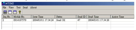
Each short message item will be assigned a unique sequence number by the program. After this message is sent out by the MT360 GSM module, the GSM module will reply a send ID to identify this message.
